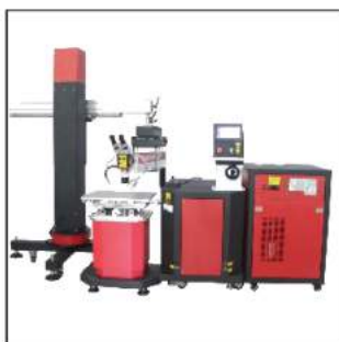
Mould Repair Laser Welding
