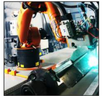
Hybrid Laser Welding
